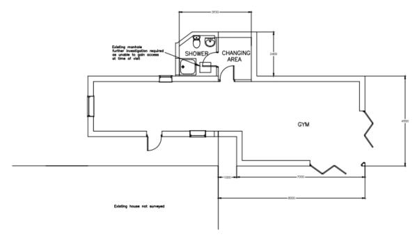
Figure 3 Proposed ground floor plan
